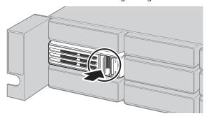
Drives without red error LEDs blinking are still on. Do not unplug or remove them.
