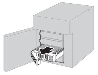
Insert the new drive into the empty slot. Slide the drive in with the locking mechanism open.
