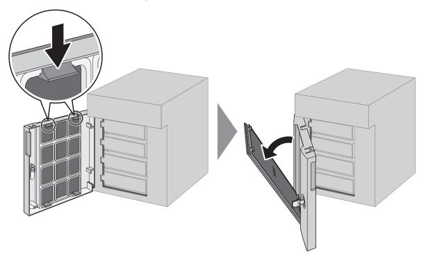
Remove the dustproof filter from the front cover and clear any dust, such as by using a vacuum cleaner.
