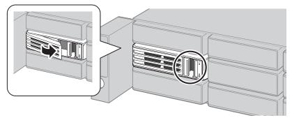
**6** When the replaced drive is recognized, the error LED will flash.
