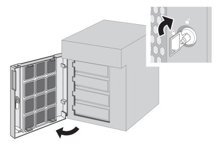
$\boldsymbol{2}$  Remove the front cover while holding the hook downward.
