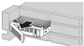
4 Insert the new drive into the empty slot. Slide the drive in with the locking mechanism open.
