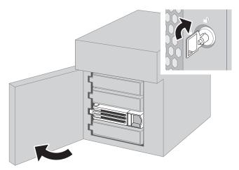
The failed drive's status LED will be glowing red. Push its unlock button and swing the lock mechanism out.
