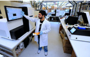
Kathy Kmonicek for The New York Times Nabil Azmay, a technician at the Cold Spring Harbor Laboratory, checks a HiSeq 2000 that reads 300 billion bases per run.
