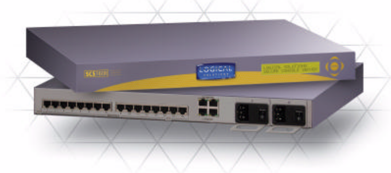
Figure 1.6 SCS160R, Secure Console Server, front and rear views
