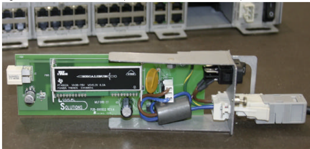
Figure 3.9 -48Vdc Power Module (shown removed from Sentinel 32)
