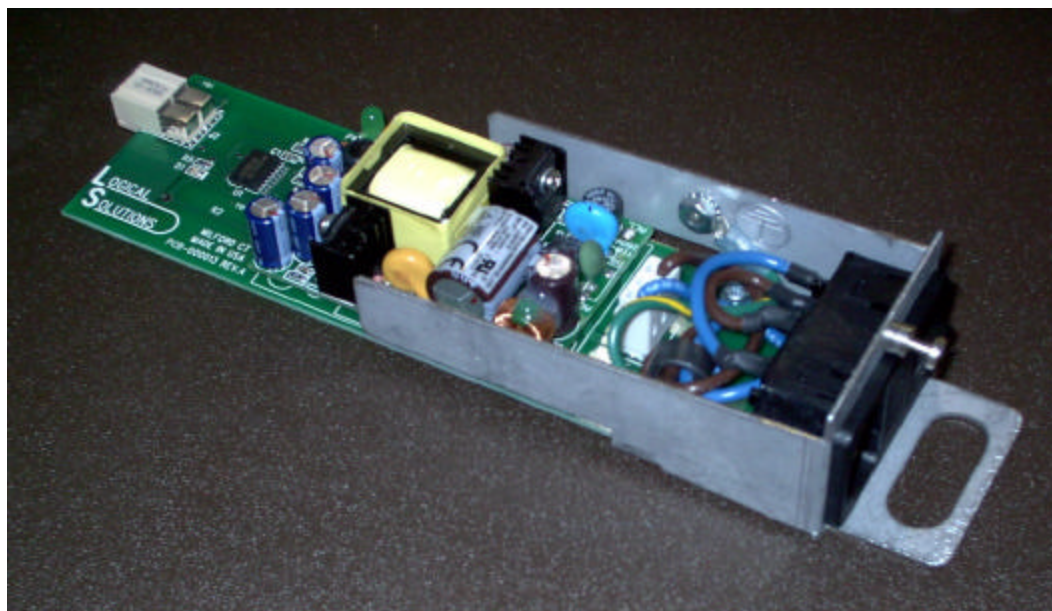
Figure 3.5 AC Power Module (shown removed from SCS320R)
