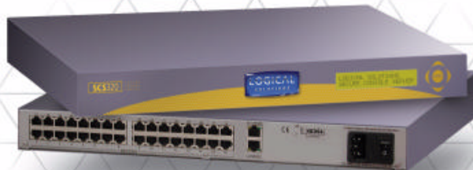
Figure 1.3 SCS320, Secure Console Server, front and rear views
